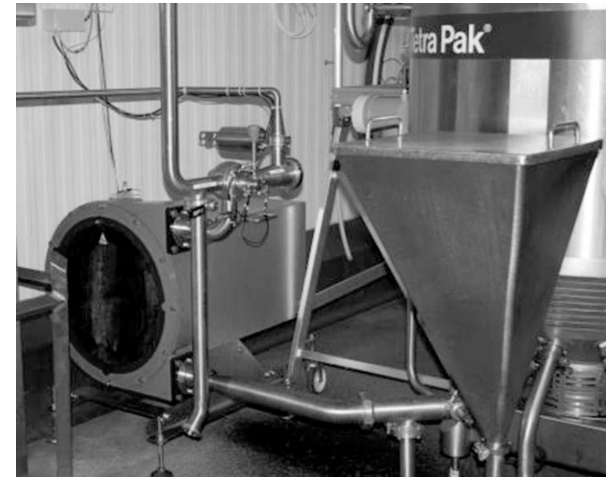
DENMARK: Transfer of salads with stuffing by food grade approved realax DFC 60 A41 with NBR-A hose.
